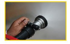
The Spray Mode offers extensive coverage and protection against radiant heat when the firefighter approaches the fire zone. Modes can be easily switched using a lever.
