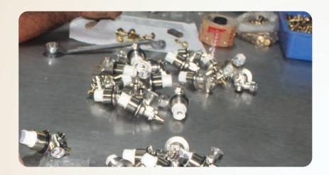
The extinguisher is then dismantled completely; cylinder is de-stressed.
