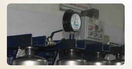
The cylinder then is made to undergo a Hydrostatic Pressure Test at 30kgf cm sq for 2 minutes to check for leaks and the burst capacity.
