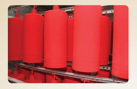
The cylinder undergoes the fresh painting process by first Static Charge Powder coating and then baking in Oven at 180 degrees for 15 minutes. This results into a super fine quality and durable new paint surface on the cylinder.
