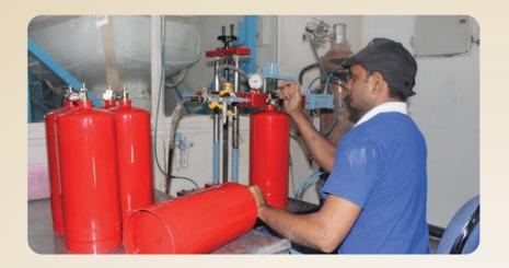
7. Fire extinguisher is charged (pressurized) with 99.99% pure nitrogen mixed with helium
