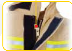
60 cm zipper on the front with quick release system, concealed by a storm flap, closes with FR Velcro fasteners.
