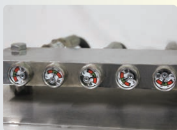
✓ Pressure Gauge Test
