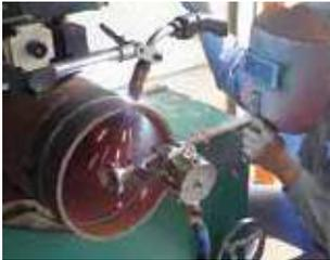
After mechanically rolling the sheet to form a cylinder shape, the two ends are seamed together by advanced welding technology - Motorised Metal Inert Gas (MIG) CO<sub>2</sub> welding.
