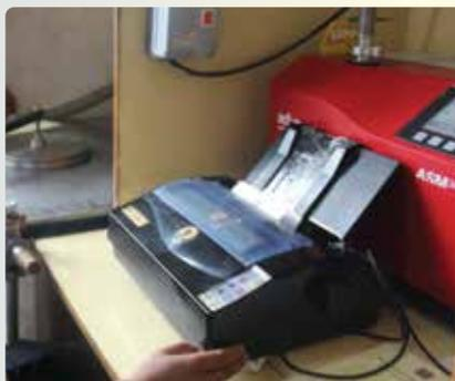
✓ The Helium Leak Detection Test: To ensure our extinguishers won't lose even a finest trace of gas or pressure throughout their service life, the container is charged with 99.99% pure nitrogen and a little helium and put into a helium sensitive machine chamber. Being lighter than nitrogen, helium leaks through the welded joints of faulty container bodes. If a trace of helium is found, the cylinder is rejected.
