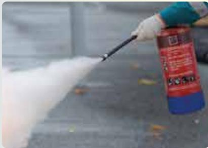
**12.** ABC Powder-based extinguishers contain highly potent MAP 50 or MAP 90 powder. The powder always remains free flowing because the cylinders are filled by an automatic machine in a dehumidified environment. Ensuring no moisture content. Silicon is further added to make the ABC Powder moisture repellent.
