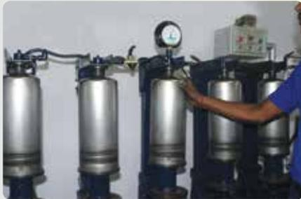
Ceasefire's production guidelines make it **mandatory to conduct specialised Hydrostatic Pressure Testing on every single container.**
