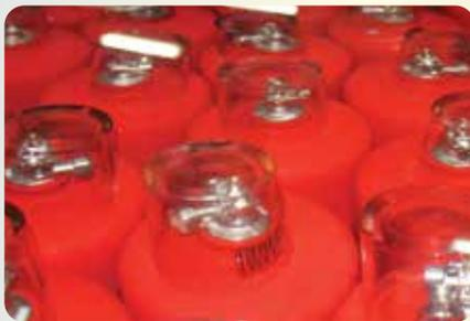
**Once the extinguisher is pressurised, it's important to check that there are absolutely no leaks.**
