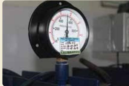
A minimum of 30 kgf/cm<sup>2</sup> pressure is exerted on the container for 2 mins. **That's 3 times more pressure than a fire extinguisher, ensuring a perfect container.**
