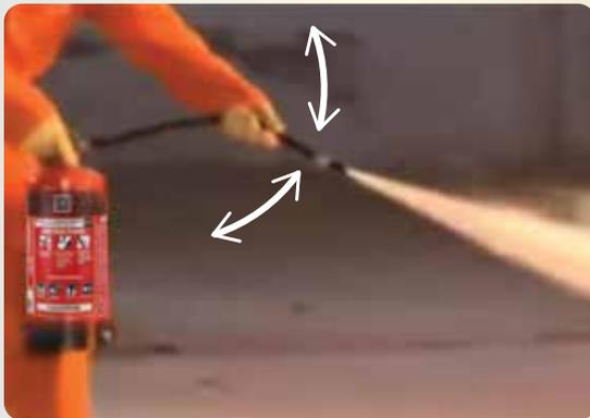
Being flexible, they can be **swiftly moved from side-to-side to fight the fire. Flexibility** at the time of activation is **vital for effective firefighting.**
