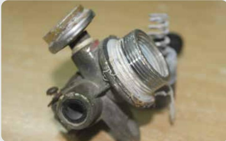
Valves most commonly malfunction because they're **forged at the wrong temperature. This makes the metal brittle**, not allowing improper integration of components and poor quality rubber O-Rings.
