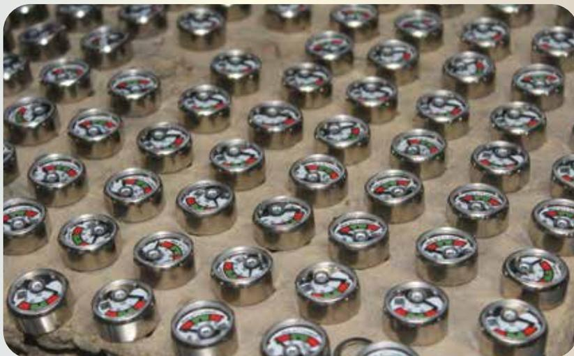
With Ceasefire Pressure Gauges, **the needle can be checked against jamming using a magnet.**
