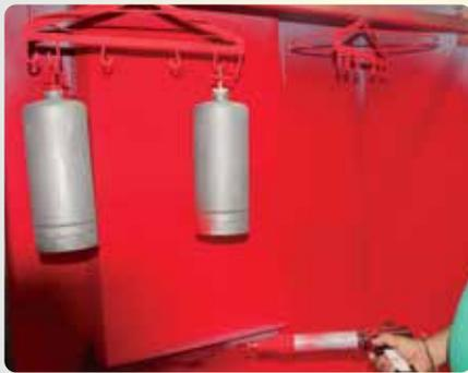
The **paint is first positively charged, and the containers, negatively** to ensure the powder coat temporarily fixes to the containers.
