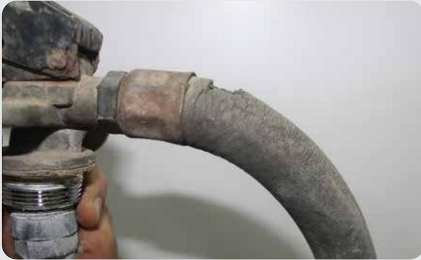
Under harsh conditions and over time, the **ordinary rubber and PVC** used to make these hosepipes **becomes brittle and starts crumbling.**
