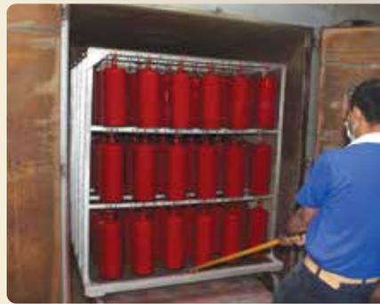
Containers are then placed inside giant ovens and baked for **15 minutes at 180°C**. The **powder particles melt and form a lustrous layer of paint.**
