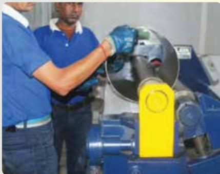
A specialised **Deep Draw process** is carried out to give the CRCA steel sheets the shape of a container.
