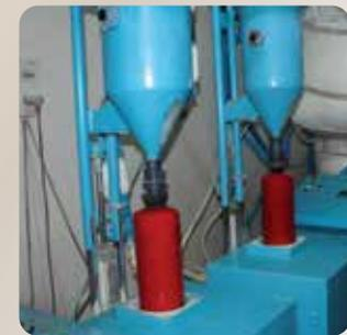
The vacuum sucks the ABC Powder into a hopper, which in turn **releases just the right amount of powder into the attached container** - allowing **no moisture in.**
