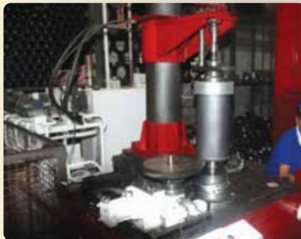
This process involves **moulding through hydraulic presses**. Three draws are made at precise tonnage of pressure.
