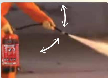
**7.** Hosepipes made of braided rubber or EPDM. They are durable, do not become brittle over time or crack; and are able to withstand the pressure when the agent is dispersed. Being flexible, they can be swept from side-to-side for effective firefighting.
