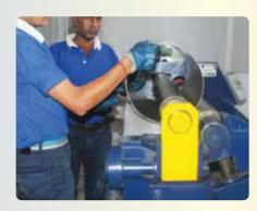
A specialised **Deep Draw process** is carried out to give the CRCA steel sheets the shape of a container.
