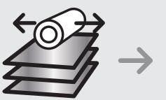
Container bodies are made by rolling flat steel sheets
