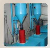
The vacuum sucks the ABC Powder into a hopper, which in turn releases just the right amount of powder into the attached container - allowing no moisture in.
