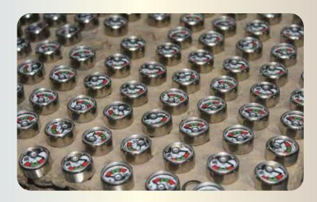
With Ceasefire Pressure Gauges, the needle can be checked against jamming using a magnet.
