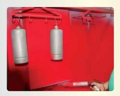
The paint is first positively charged, and the containers, negatively to ensure the powder coat temporarily fixes to the containers.
