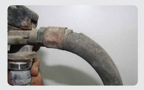
Under harsh conditions and over time, the **ordinary rubber and PVC** used to make these hosepipes **becomes brittle and starts crumbling.**
