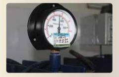
A minimum of 30 kgf/cm<sup>2</sup> pressure is exerted on the container for 2 mins.
