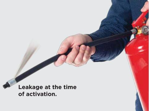
Most industry players use **ferrules made of iron** to attach the hosepipe to the extinguishers. This **iron** rusts quickly, losing its strength, and giving way at the time of activation and discharge.
