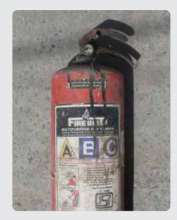
Spray painting is the most common process, resulting in an inferior grade finish, scratches during installations and rapid deterioration.
