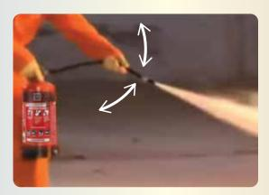
Being flexible, they can be swiftly moved from side-to-side to fight the fire. Flexibility at the time of activation is vital for effective firefighting.
