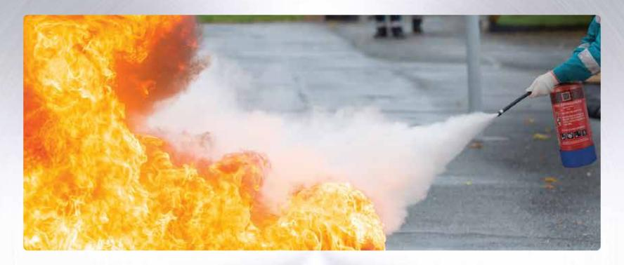
The actual potency of a fire extinguisher comes from the extinguishing agent used in it. Every other component in the extinguisher is designed and created to ensure that this agent gets delivered from the extinguisher to the fire effectively. It is solely the agent's job to actually take on, and put out the flames.
