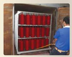
Containers are then placed inside giant ovens and baked for 15 minutes at 180°C. The powder particles melt and form a lustrous layer of paint.
