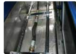
✓ Hosepipe Burst Pressure Test
