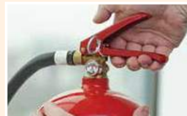
Press the trigger firmly to activate the fire extinguisher.
